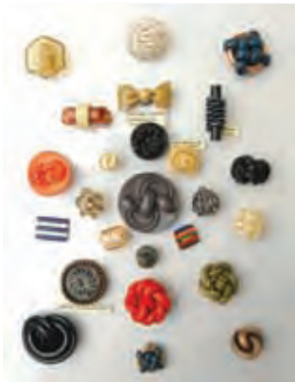
Extruded celluloid buttons are made by using the material to pipe and swirl into molds. These buttons were made in the 1920s and '30s.
